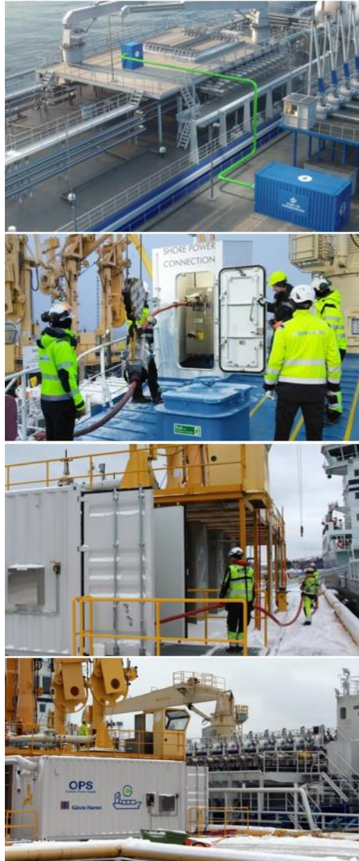
FLYING PLUG avoids waste of time, use of on board cranes, and intense labour compared to IEC solution
