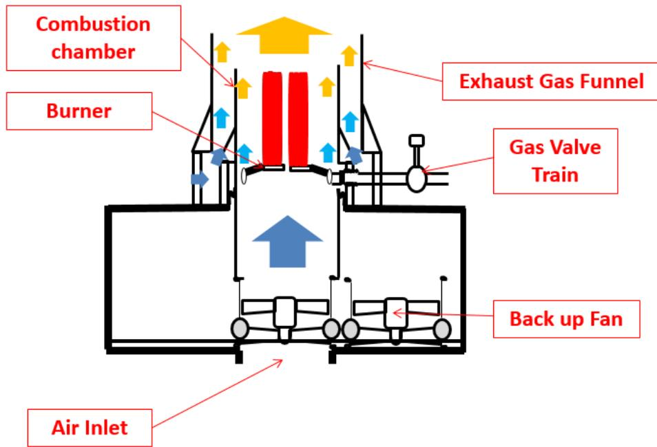
*ECOFLARE main Components and architecture (Patent pending)*
